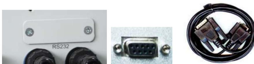
Fig. 10 RS232 serial port and special RS232 cable
